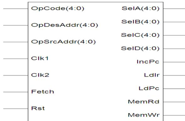
Fig.11: Block Diagram of Control unit
